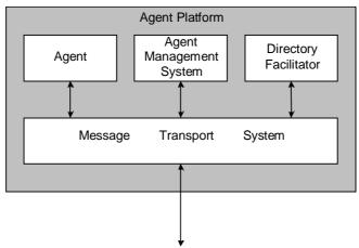
Figure 1 - Reference architecture of a FIPA Agent Platform
